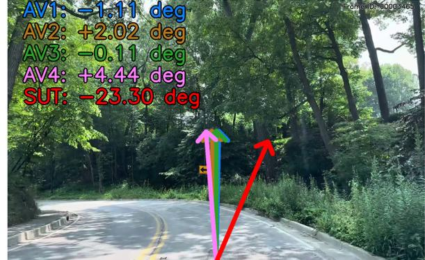
Fig. 1: DIFFTEST4AV identifies this input image as one causing a high-impact failure: over 90% confident the SUT response to that image is an outlier when compared with the reference systems, and causes a 20° output difference. SUT steering (red line) causes the vehicle to turn off-road.
